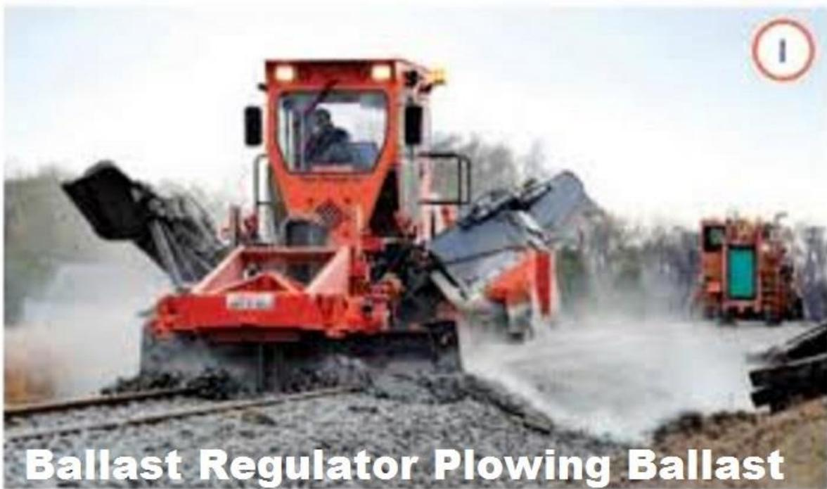
**Ballast Regulator Plowing Ballast**
